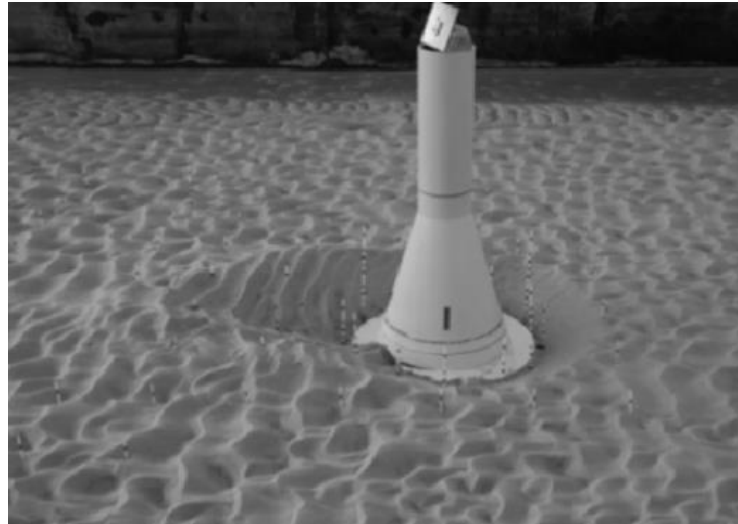
Figure 7: Form of the equilibrium scour hole developed around a conical GBS foundation in a scaled model test for Thornton Bank (Bolle et al., 2010).
